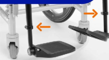
The footrest height of the swing-away legrests can be adjusted by loosening the bolts with an Allen key no. 5 and lowering the footrest.
