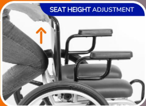
Push the seat max. one pin up on the front of the seat comparing to the rear, to create an angular adjustment. Replace the pins at front and push the rear down (one hole lower) and replace the pins at the rear.
